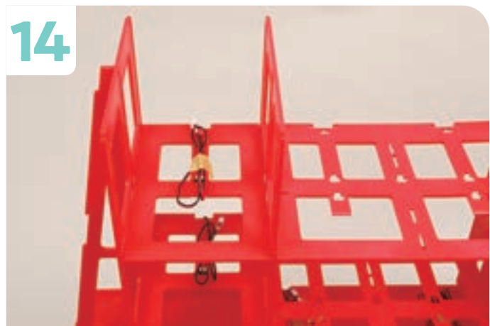
Pull the cable taut and lead it to the top of the Shelving Board, then bundle it out of the way and temporarily secure it in place with masking tape.
